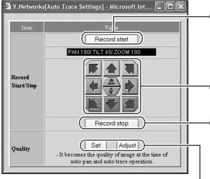
Press Record start to display the [Record Start Confirmation Screen]. Memorization of Auto Trace will start upon clicking OK and subsequent Pan/Tilt as well as Zoom operations will be stored. (Approximately 30 seconds)
